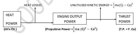
Propulsive power available to propel aircraft forward is propulsive power and actual power available to propel aircraft forward is thrust power.
