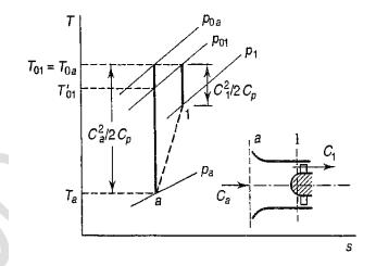
The main function of intake is to minimize the pressure loss upto the compressor phase while ensuring that the flow enters the compressor with uniform pressure and velocity.
